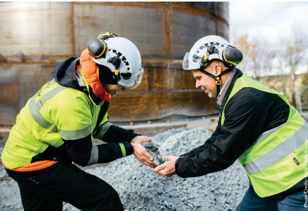
In Pornainen, Finland, 2,000 tonnes of crushed soapstone is being used to store clean energy in the form of heat
